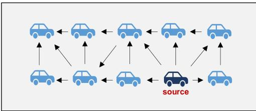
The data relaying capabilities of CVs can be also a savior in the cases of **emergencies** or **natural disasters** when other communication infrastructures are down because of their reliance on communication wires. In such cases, vehicle-based information dissemination can be used for relaying critical data to/from the crisis management authorities, and for guiding emergency vehicles and staff through the best available routes.
