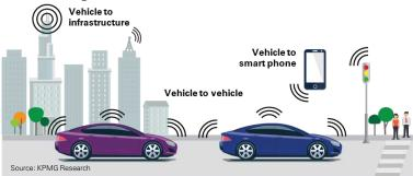
Modern car connectivity technologies permit communication on multiple fronts: pedestrians (V2P), infrastructure (V2I), other vehicles (V2V), cloud service (V2C), and all vehicles and transportation infrastructure (V2X).<sup>10</sup> Most modern vehicles are connected on one of these fronts through features such as lane adjustments, car condition alerts, and Geographic Positioning Systems.
